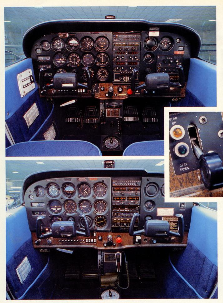
The landing-gear lever (inset) and propeller control are the primary differences between a 172RG panel (left) and that of a 1980-vintage fixed-gear model (below left).
